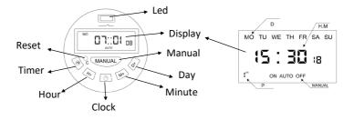
$\checkmark$  To start, press the RESET button. Set the local time by pressing the CLOCK, and the D+, H+ or M+ buttons to adjust the current local time.
